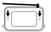
(When turning the unit over, be careful not to lose the two screws as they might fall out.)
